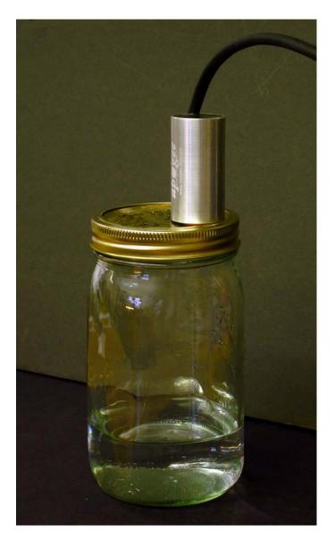
**Figure 4:** Apogee  $O_2$  sensor mounted in a sealed chamber over water. For measurements in environments where the RH = 100 %, sensors should be calibrated in conditions where the RH = 100 % in order to account for any humidity effects on sensor electronics.
