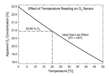
temperature. As temperature changes, relative oxygen concentration remains constant at 20.95 %, but an apparent oxygen change is measured if the temperature correction is not applied to relative measurements. It is assumed the sensor was calibrated at 20 C, and the solid line shows how the apparent relative oxygen concentration is dependent on temperature.
