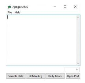
When the ApogeeAMS software is first opened, it will show a blank screen until communication with the meter is established. If you click "Open Port" it will say "connection failed."
