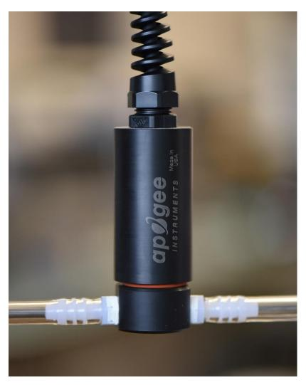
Apogee oxygen sensors are resistant to 2.7 G of shock, but vibration may influence sensor sensitivity and should be minimized.
