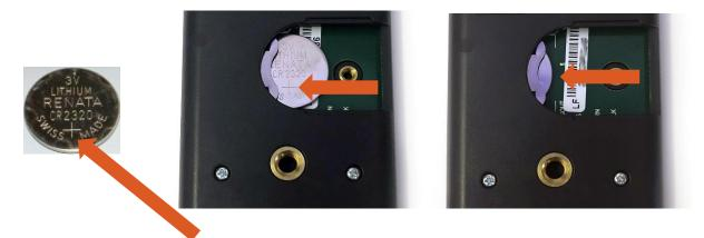
The positive side (designated by a "+" sign) should be facing out from the meter circuit board.
