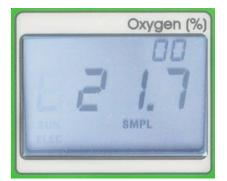
The LCD display consists of the total number of logged measurements in the upper right hand corner, the real-time percent oxygen concentration in the center, and the selected menu options along the bottom.
