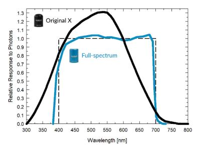
Mean spectral response measurements of six replicate Apogee SQ-100X (original X) and MQ-500 (full-spectrum) series quantum sensors. Spectral response measurements were made at 10 nm increments across a wavelength range of 300 to 800 nm with a monochromator and an attached electric light source. Measured spectral data from each quantum sensor were normalized by the measured spectral response of the monochromator/electric light combination, which was measured with a spectroradiometer.
