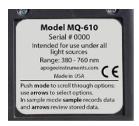
Sensor model number and serial number are located on a label on the backside of the handheld meter.
