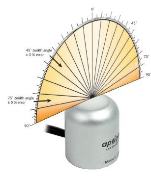
Directional, or cosine, response is defined as the measurement error at a specific angle of radiation incidence. Error for Apogee MQ-600 series ePAR Sensor is approximately  $\pm 2$ % and  $\pm 5$ % at solar zenith angles of 45° and 75°, respectively.
