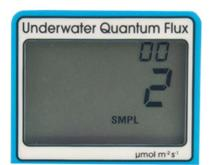
The LCD display consists of the total number of logged measurements in the upper right hand corner, the real-time PPFD value in the center, and the selected menu options along the bottom.
