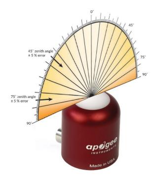
Directional, or cosine, response is defined as the measurement error at a specific angle of radiation incidence. Directional error for Apogee S2 series red - far-red sensors is approximately  $\pm$  2 % and  $\pm$  5 % at solar zenith angles of 45° and 75°, respectively.
