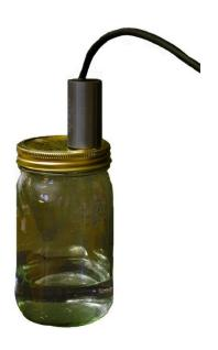
Apogee oxygen sensor mounted in a sealed chamber over water. For measurements in environments where relative humidity is 100 %, sensors should be calibrated in conditions where relative humidity is 100 % in order to account for any humidity effects on sensor electronics.
