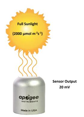
Example of photon flux density measurement with an Apogee model SQ-610 ePAR Sensor. Full sunlight yields a photon flux density on a horizontal plane of approximately 2000  $\mu mol~m^{-2}~s^{-1}.$  This yields an output signal of 20 mV. This signal is converted to photon flux density by multiplying by the calibration factor of 100  $\mu mol~m^{-2}~s^{-1}$  / mV.
