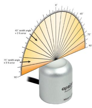
Directional, or cosine, response is defined as the measurement error at a specific angle of radiation incidence. Error for Apogee SQ-600 series ePAR Sensor is approximately  $\pm$  2 % and  $\pm$  5 % at solar zenith angles of 45° and 75°, respectively.
