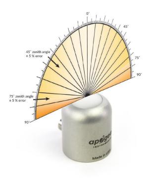
Directional, or cosine, response is defined as the measurement error at a specific angle of radiation incidence. Error for Apogee SQ-600 series Quantum Light Pollution Sensor is approximately  $\pm 2$  % and  $\pm 5$  % at solar zenith angles of 45° and 75°, respectively.
