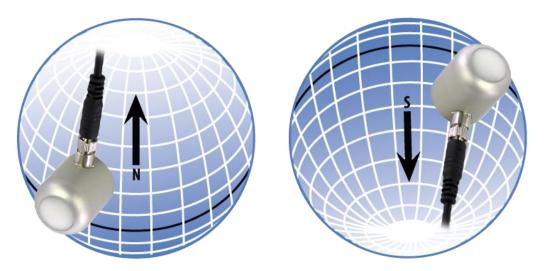
In addition to orienting the cable to point toward the nearest pole, the sensor should also be mounted such that obstructions (e.g., weather station tripod/tower or other instrumentation) do not shade the sensor. **Once mounted, the blue cap should be removed from the sensor.** The blue cap can be used as a protective covering for the sensor when it is not in use.
