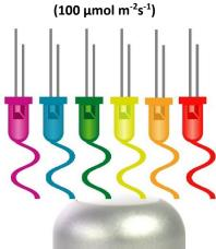
Example of photon flux density measurement with an Apogee model SQ-644 Quantum Light Pollution Sensor. The LED in this example Full yields a photon flux density on a horizontal plane of 100  $\mu mol\ m^{-2}\ s^{-1}.$  This yields an output signal of 12 mA. This signal is converted to photon flux density by subtracting the 4.0 mA offset and then multiplying by the calibration factor of 12.5  $\mu mol\ m^{-2}\ s^{-1}$  / mA
