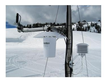
Top left: SP-230 Heated Pyranometer
