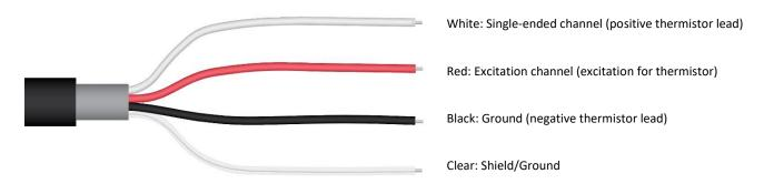
Wiring for ST-100 Serial Numbers range 0-2724, ST-110 Serial Numbers range 0-2724, and ST-200 Serial Numbers range 0-1351
