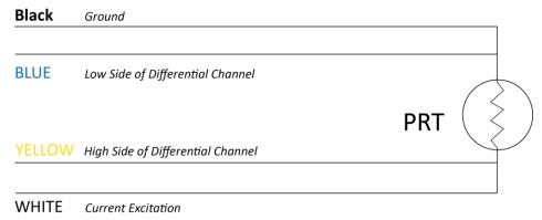
Note: as shown in the schematic, the 4-wire PRT can be directly measured. The black and blue wires are electrically connected to one side of the PRT while the yellow and white wires are electrically connected to the other side of the PRT.
