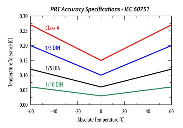
Accuracy for multiple classifications of PRTs across a temperature range of -60 to 60 C. Temperature tolerance specifications (y axis) are defined by International Electrotechnical Commission (2017).
